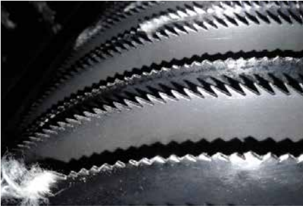
Fig. 1. The operational state of the saw blades after 168 hours of work, set by alternation (with hardened and non-reinforced teeth) on gin 5DP-130
